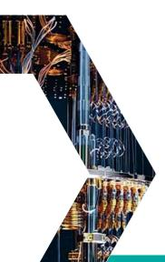
The LUMI-Q consortium's quantum computer, named VLQ, will be based on superconducting qubits and will feature a unique star topology. This topology minimises the number of so-called swap operations, enabling the execution of highly complex quantum algorithms. The system will feature 24 physical qubits connected to a central resonator.
