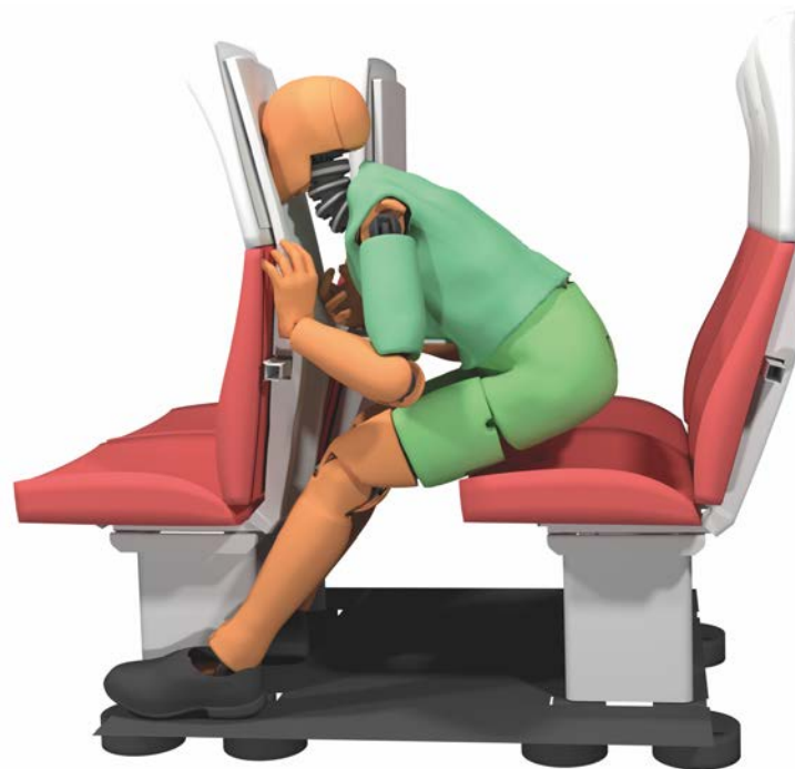
Crash test simulations of new seats for improved passive safety and comfort of passengers in railway traffic, research project awarded the HiPEAC Technology Transfer Award
